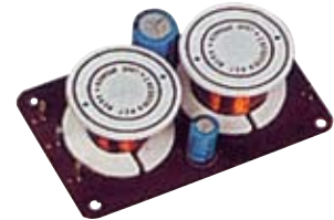
GT2-1069 (SH611) 100W 2WAY 12dB/OCT FREQ.: 2.5KHz IMPEDANCE: 8 \Omega
