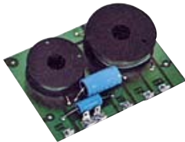
GT2-1067 (SH606) 100W 3WAY 6dB/OCT FREQ.: 1k~5KHz IMPEDANCE: 8/4 \Omega
