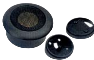
GT2-1044 (TW110) Satellite Kevlar Tweeter 4 ohm 15W 25mm Kapton Voice coil 25x3.5mm NdFeB Magnet
